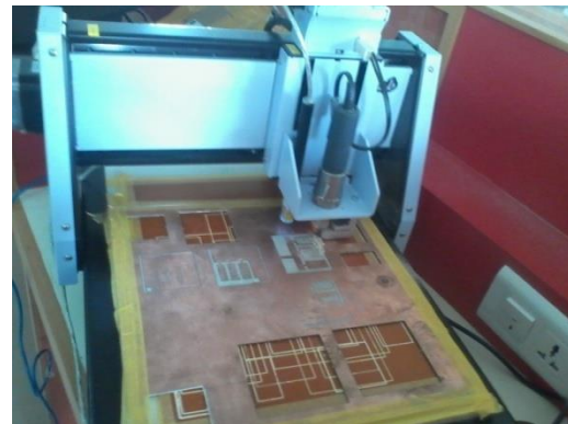
Fig.2. Fabrication of proposed antenna using ELEVEN LAB
