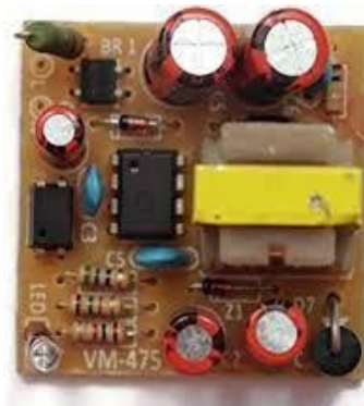
Fig. 5: Power Supply Board
