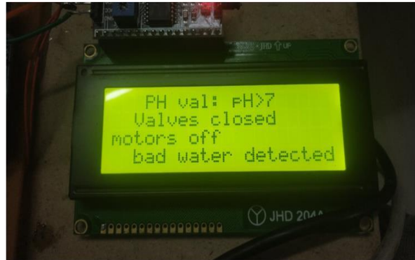
Fig 4.4: Display of Polluted water detected
