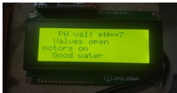
Fig 4.3: Display of Normal Water Detected
