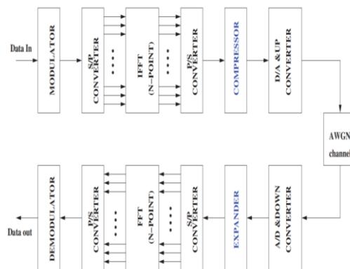
Fig. 6. Block diagram of \mu law companding
