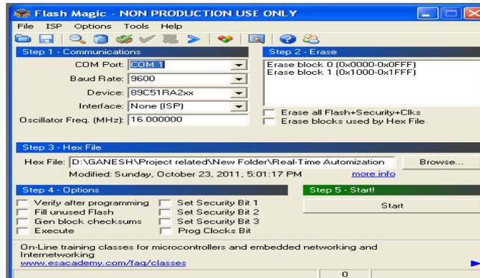
Fig. 10. Dumping of the code into Microcontroller
