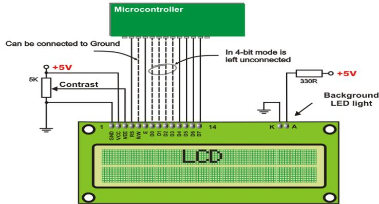
Fig. 4. Interfacing of LCD to a micro controller
