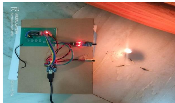
Fig.9: Fire with far distance to sensor
